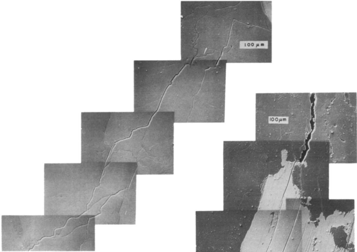
Fig. 4. Sub-parallel array of en-échelon cracks in plagioclase grain of GC-2. Note that a high proportion of the healed cracks have not re-opened. Maximum compression was vertical.
